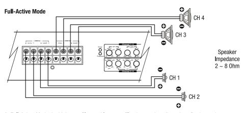
At Full-Acitve Mode the high pass filter and low pass filter have to be adjusted confirming to the used midrange speaker and tweeter. **Therefore contact you specialist dealer.**
