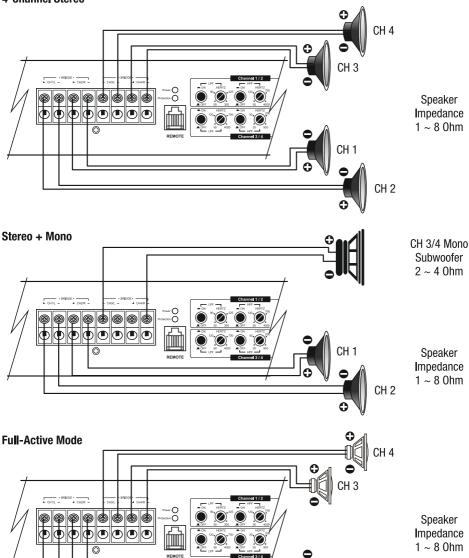
At Full-Acitve Mode the high pass filter and low pass filter have to be adjusted confirming to the used midrange speaker and tweeter. **Therefore contact you specialist dealer.**
